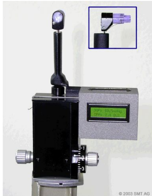
Fig. 9 (below) Dynamic Contour Tonometer constructed by the authors (experimental device). Custom-built contour tonometer tip is mounted on the base of a Goldmann Tonometer, which is set to provide 1 gm appositional force. Pressure measured by built-in sensor is read from LCD display and may be transferred to a connected PC.
